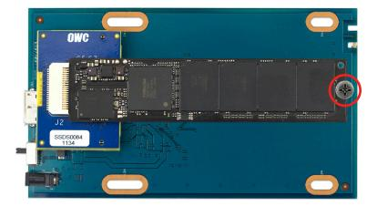
Insert the included 8-32 Phillips head screw into the nylon standoff to secure your Apple flash storage module into the bridge card.
